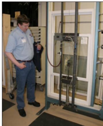
Window Worlds constant force balance systems have been tested for up to 15,000 consecutive openings and closing without failure. This is a lifetime of openings and closings. If the stainless steel balance does fail, it can be easily replaced.
