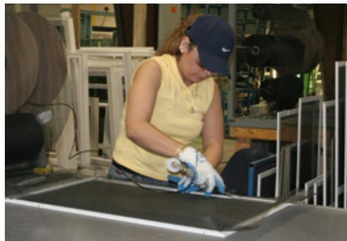
Screens are made out of rigid extruded aluminum and have a powder coat paint finish. The spline (the part that holds the screen in) is on the inside so it doesn't deteriorate over time and it has a nice clean look.
