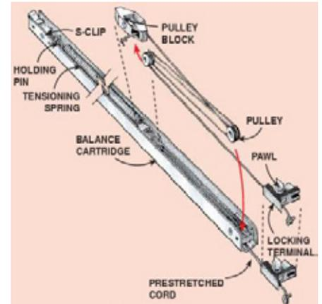
Spring & Rope or Block & Tackle balance systems are more prone to failure. When they do fail, they are nearly impossible to replace without cutting or taking the window frame apart.
